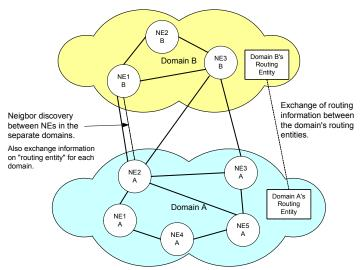
Fig. 6. Intracarrier intervendor routing domains.
