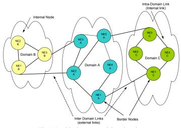
Fig.1. Partitioning a network into domains.
